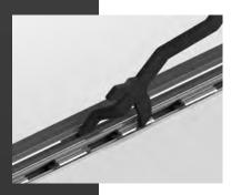
Insert the nipple at the centre tip of the tensioning tool into the profile groove above the tensioning channel. Press down the left or right tip of the tensioning tool to engage the flex holder in the teeth of the tensioning channel and tension the fabric. Then seal the tensioning channel with the cover profile and use screws to prevent it from springing off unintentionally.
